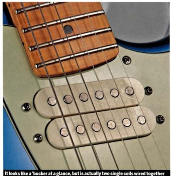
It looks like a 'bucker at a glance, but is actually two single coils wired together
